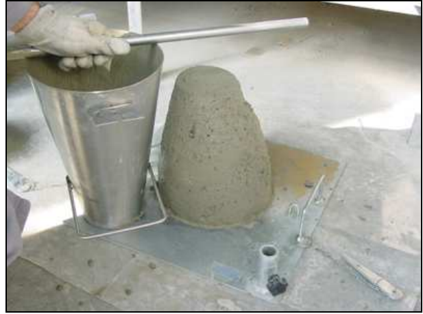
Slump S2 - 50-90mm
