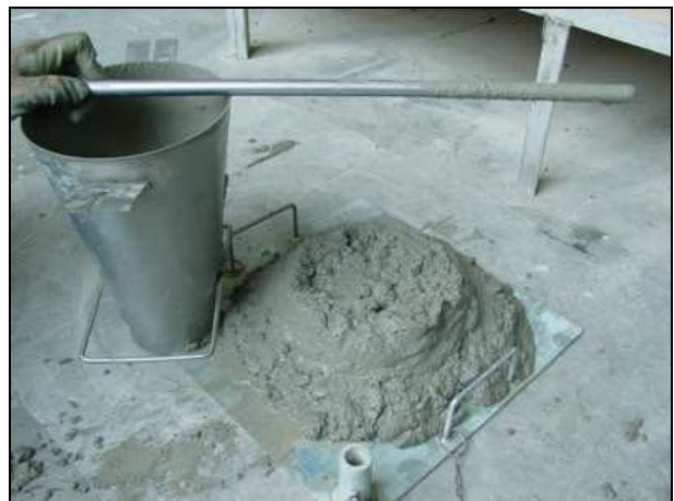
Slump S4 - 160-210mm
