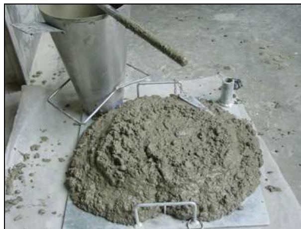
Slump S5 - > 220mm
