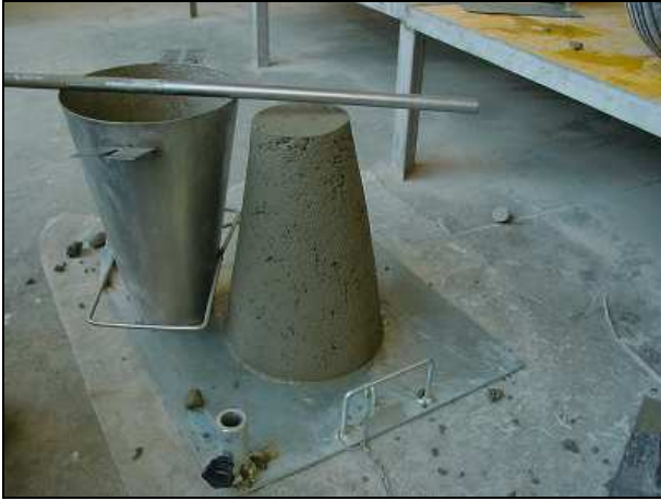
Slump S1 - 0-40mm
