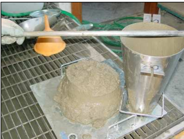
Slump S3 - 100-150mm
